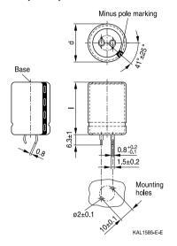
Snap-in terminals, length ( $6.3\pm1$ ) mm. Also available in a shorter version with a length of (4.5-1) mm. PET insulation is marked with label "PET" on the sleeve. Safety vent on the base.
